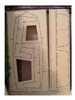
Temporary frame front internal 12mm Temporary frame rear internal 12mm
